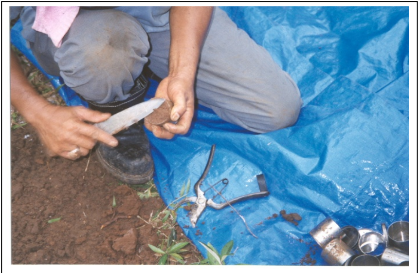
Figure 10. Disposal of the remaining soil from the ring soil sampler (Source photo: JICA, 2002).
