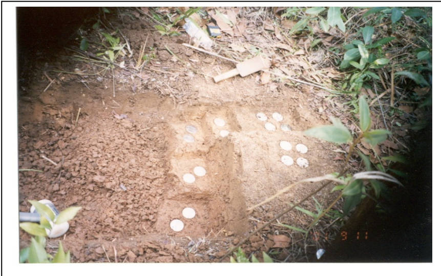
Figure 9. Position ring soil sampler (Source photo: JICA, 2002).
