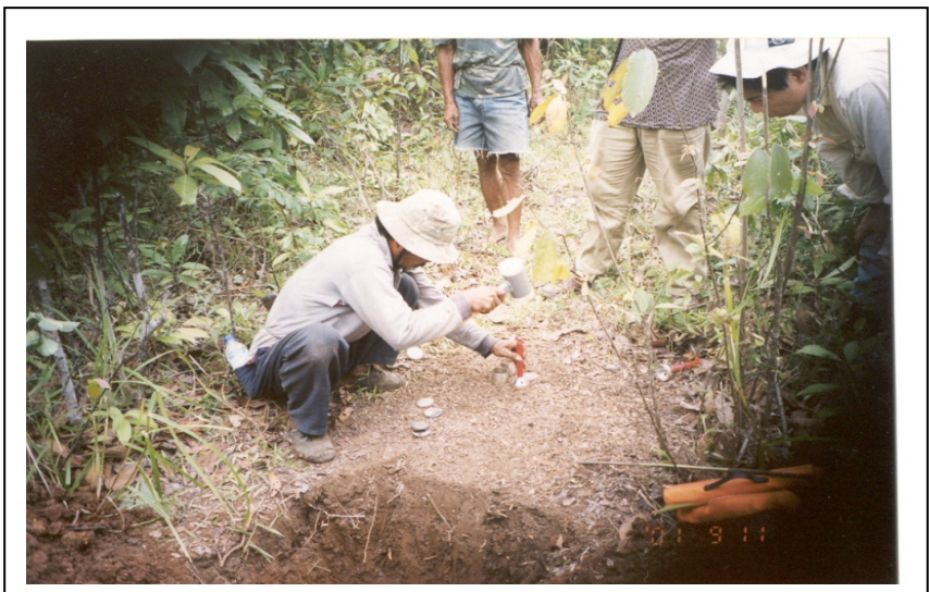
Figure 8. The placement of ring soil sampler on the soil surface (Source photo: JICA, 2002).
